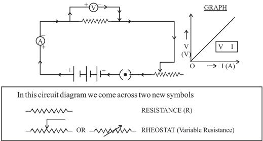
**Ohm's Law** He stated that the electric current flowing through a conductor is directly proportion at to the potential difference across its ends, provided the temperature remain constant
