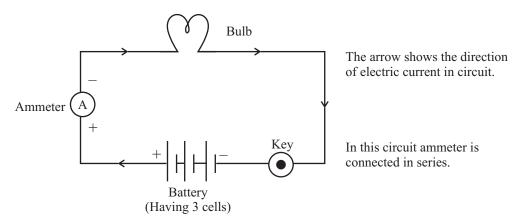
**The electron can only flow when there is difference of electric pressure.** For example "water flowing through a tube" It is only possible when there high pressure at one side and low at another side, then it will move from high pressure to low pressure.
